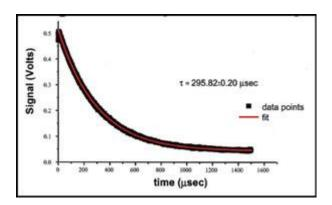
This graph depicts the concept of ring-down decay within the cavity after the laser source is shuttered. As the laser light bounces back and forth between the ultra-high reflective mirrors, the sample species absorbs the light energy until it's all gone.
